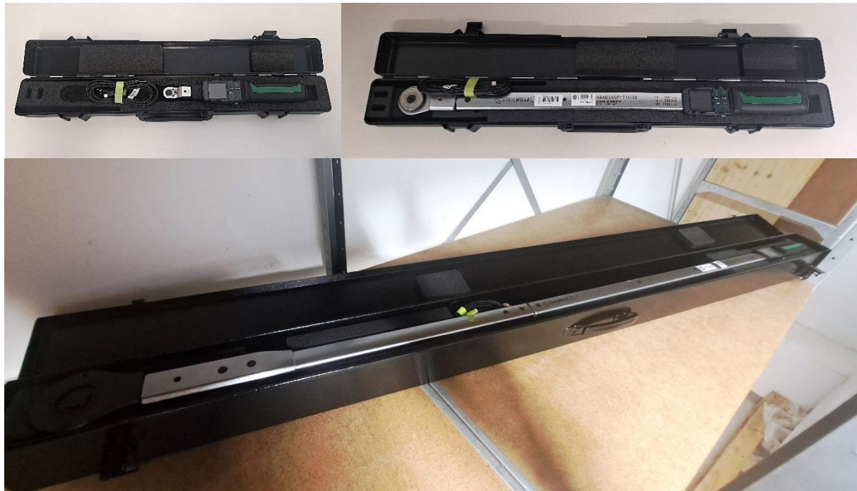
Figure 1: Top left: KG 1: 10 Nm torque wrench. Top right: KG 2: 200 Nm torque wrench. Bottom: KG 3: 1000 Nm torque wrench
