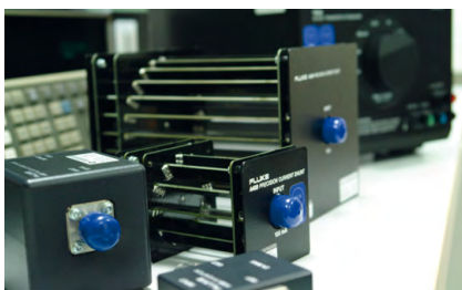
Reference standards for alternating current power
