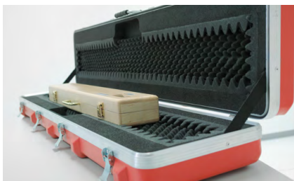
Special transport boxes equipped with shock-, tilt- and temperature indicators for the transport of resistance thermometers and fixed point cells.
