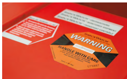
Special transport boxes equipped with shock-, tilt- and temperature indicators for the transport of resistance thermometers and fixed point cells.
